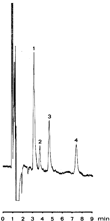
Fig. 2. High-performance liquid chromatogram of 1000 \mu l of tap water spiked with 10 \mu g/l of 4-nitrophenol (1), 2-nitrophenol (2), 2,4-dinitrophenol (3) and 2,4-dinitro-2-methylphenol (4). Column, Li-Chrosorb RP-18, 5 \mu m (250 \times 4.6 mm I.D.); mobile phase, 30 ml of PIC-A reagent in 1 l of water-methanol (55:45); flow-rate, 1 ml/min; absorption, 405 nm; a.u.f.s., 0.005; recorder setting, 10 mV.
